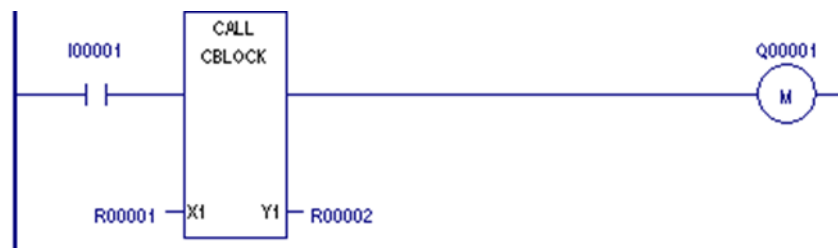
Figure 6: Invoking a C block from Ladder Program
